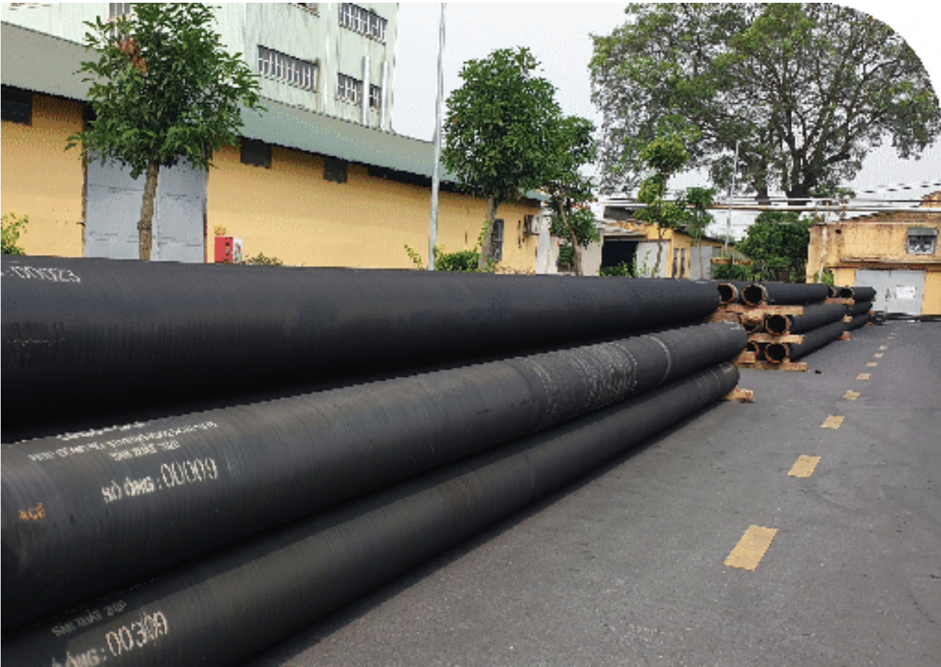
Composite insulation coating for undersea oil pipelines
