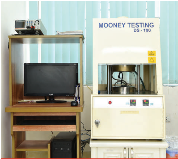
Mooney Testing Machine Check rubber viscosity
