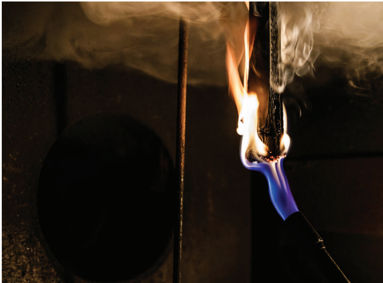
Fire resistance test according to ISO 340
